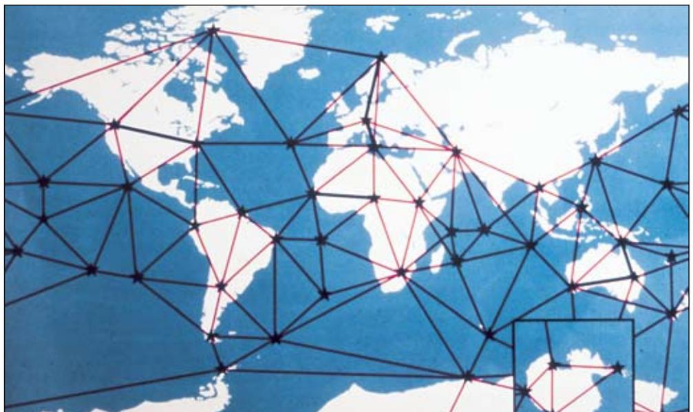
**FIGURE 1** BC-4 Satellite Triangulation Network.
